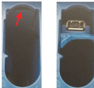
Figure 2-3 Push the cover ( left ) and pull out the hidden USB 2.0 port ( right )
