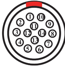
Figure 6-2 Alarm and I/O LEMO connector (contact view)
