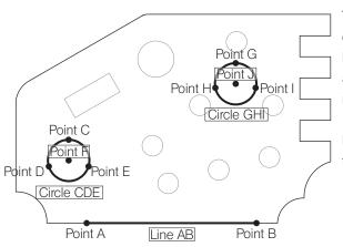
The distance between 2 points, the coordinate difference X and the coordinate difference Y can be measured by specifying the line AB. By specifying the circle CDE and the circle GHI, the coordinate F and J of the center point, radius and diameter of each circle can be measured.
