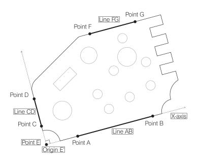
By specifying the line AB and line CD, the distance between 2 points, the coordinate difference X and the coordinate difference Y of each line can be measured.
