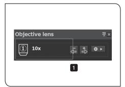
Confirm that the magnification of the objective in the [Objective lens] window is same as the magnification of the objective to be used.
