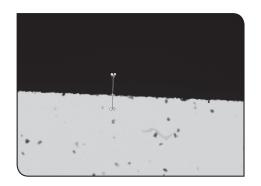
7 Drag the displayed line tool to determine the measurement points.
