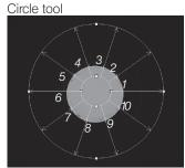
The input point positions are in the order of Input point 1, Input point 2, Input point 3 and so forth rotating counterclockwise from the 3 o'clock position.
