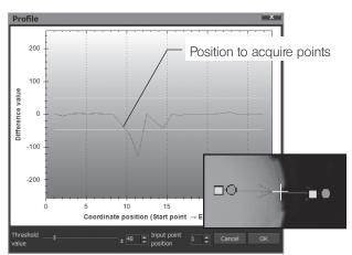
The position where the profile and the difference value are intersected is acquired as an edge point. The edge point position can be adjusted finely by changing the threshold settings.
