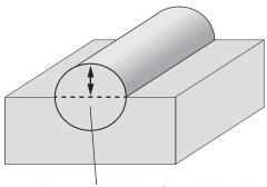
Measure the height of the raised work Distance between circle and line (upper)
