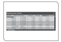
The first round of measurement results are displayed in [Sample 1] and measurement results after the second round are displayed in [Sample 2]....[Sample n].
