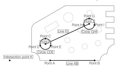
The distance between 2 points, the coordinate difference X and the coordinate difference Y can be measured by specifying the line AB.
