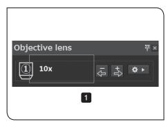
Confirm that the magnification of the objective in the [Objective lens] window is same as the magnification of the objective to be used.
