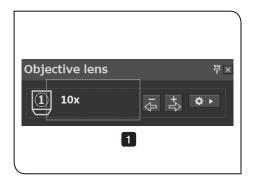
1 Confirm that the magnification of the objective in the [Objective lens] window is same as the magnification of the objective to be used.
