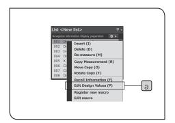
When you right-click on the measurement items in the [List] window and select [Edit design values] a in the menu displayed, you can edit the design values or tolerance values of these measurement items. Refer to "Setting design values and Excel® transfer data of measurement items" (page 99) for details.
