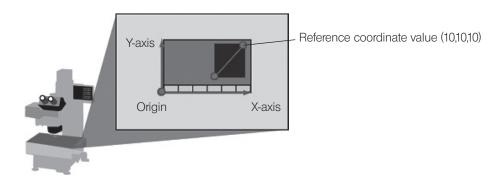
If the alignment is set, it is not necessary to place the measurement object parallel to the stage.
