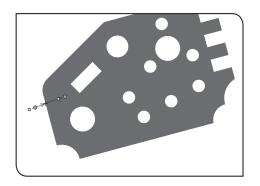
A line is created based on the clicked points, and then, one edge is detected.
