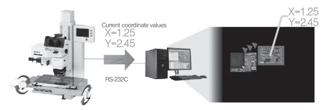
2. When the acquisition button is clicked, the current field of view is stitched to the wide range image. As the images are stitched based on the coordinate values, images can be stitched accurately.
