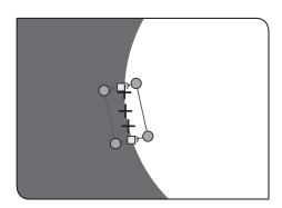
O If the circle you are measuring is large and cannot fit in the live image, the circle tool cannot detect the edge of the circle. If this
