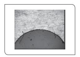
8 Move the stage to place the point C in the center of the live image.
