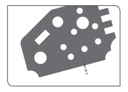
A line is created based on the clicked point, and then, one edge is detected.
