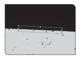
7 Drag the multipoint tool or average point tool displayed to determine the measurement points.
