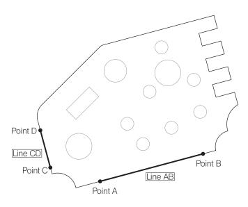
The line AB is created with the point to point measurement.
