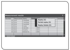
Or right-click on the measurement value number in the [Measurement results] window, and select [Replay] in the menu displayed.
