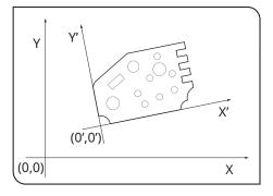
Alignment is a function to set a new origin (0',0') and the coordinate system (aligned coordinates X'Y') by the software, separately from the reference coordinate system (counter coordinates XY).
