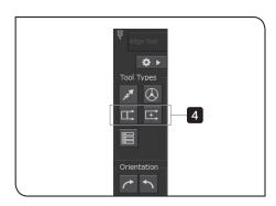
4 Click the (Multipoint tool) button of the (Average point tool) button in [Tool types].
