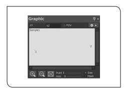
Refer to "Step 1) Get the counter data." (page 74), and acquire the coordinate data of 2 points on the X-axis in the direct measurement.
