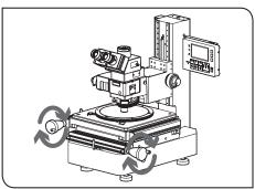
2 Move the stage of the microscope and match the cross line of the live window with the first input point.
