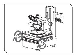
2 Move the stage of the microscope and match the cross line of the live window with the first input point.
