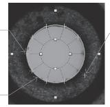
Points shown with the cross hairs in gray are the detection points outside of the effective  $\sigma$  value range. Therefore, they are not reflected to the input points. (The color can be changed by setting.)
