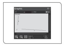
Recall the coordinate data in the order of the line AB and line CD. The intersection point E between the line AB and the line CD is created.
