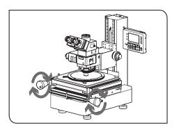
2 Move the stage of the microscope and match the cross line of the live window with the input point.
