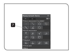
7 Click the (Intersection between line and line) button in the [Measurement items] window.
