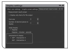
The display of the intersection angle B changes depending on the setting of [Calculation result screen settings].
