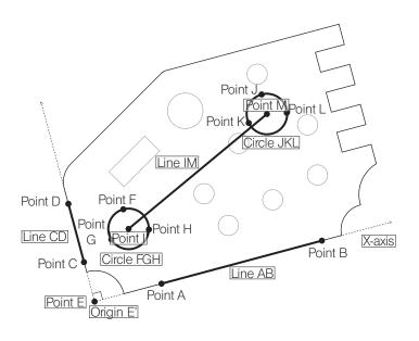
By specifying the line AB and line CD, the distance between 2 points, the coordinate difference X and the coordinate difference Y of each line can be measured. The intersection point E calculated from the line AB and the line CD is set as the origin of the aligned coordinate system.
