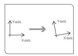
The X- and Y-axis on the live image tilt along with the X-axis of the aligned coordinate system.
