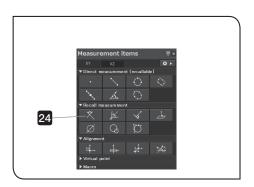
Click the (Intersection between line and line) button in the [Measurement items] window.
