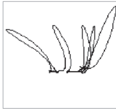
Figure 5-182 An example of an ECT absolute signal response
