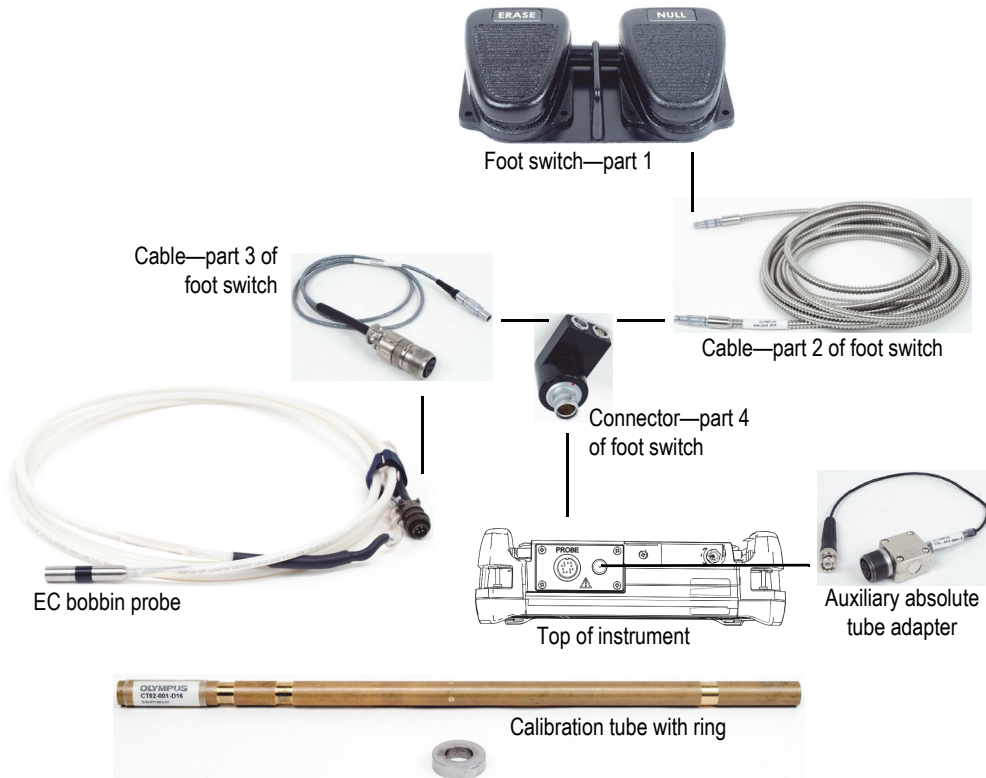
Figure 5-135 Materials—dual frequency for heat exchanger tubing
