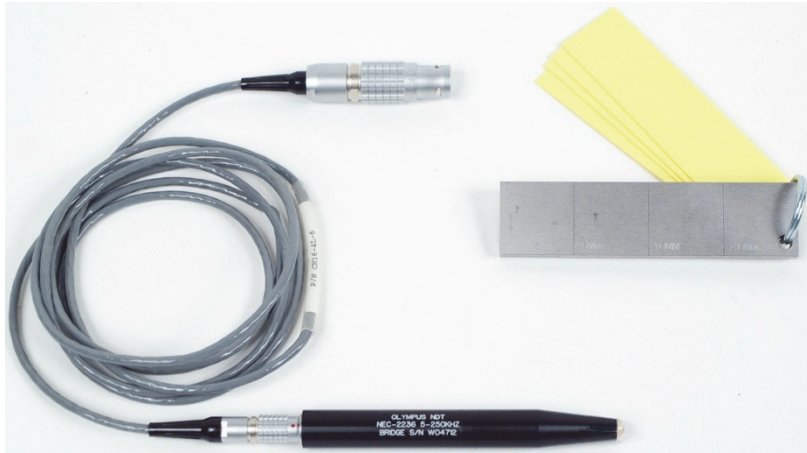
Figure 5-40 Materials—paint thickness on ferromagnetic material
