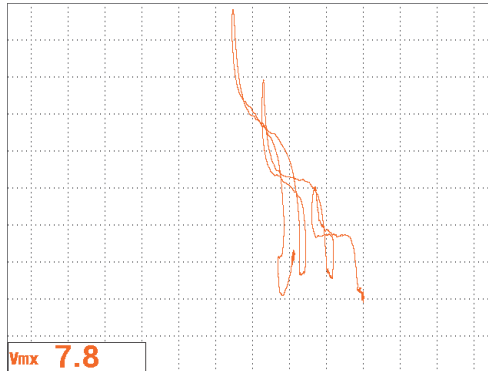
Figure 5-112 The corrosion-defect scan result
