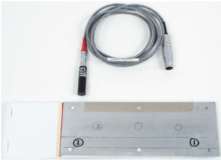
Figure 5-97 Materials—dual frequency for corrosion
