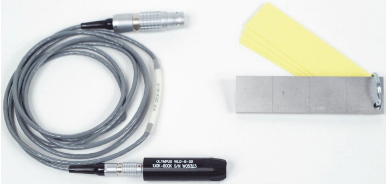
Figure 5-30 Materials—welds on ferromagnetic material
