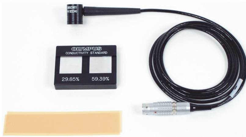
Figure 5-47 Materials—conductivity and non-conductive coating thickness
