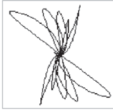
Figure 5-155 An example of an ECT differential signal response
