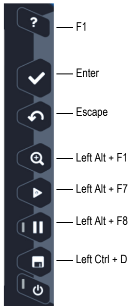
Figure 10-4 OmniScan X3 unit shortcuts
