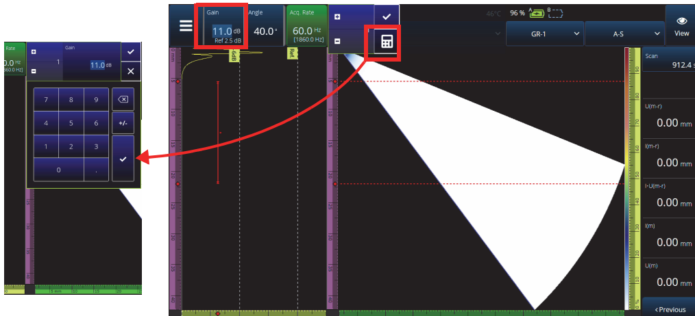
Figure 2-10 Parameter adjustment using up/down arrows or keypad
