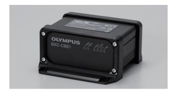
Extension control box that controls the auto focus sensor
