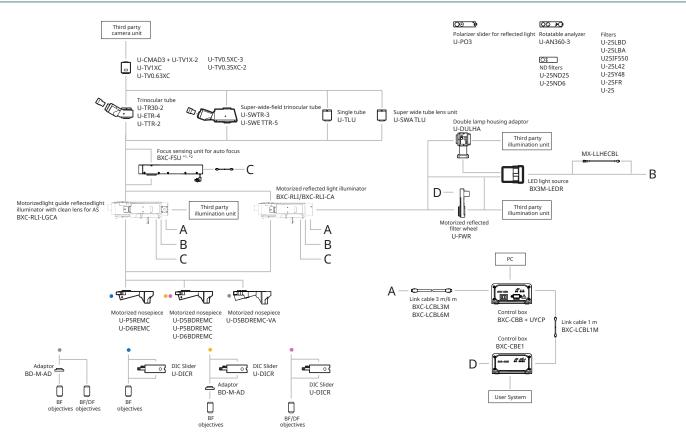
\*1 The BXC-FSU can be connected directly to the BXC-CBB to use auto focus with a manual illuminator. In this case, please note that the BXC-CBB cannot control the BX3M-LEDR without the BXC-RLI. If you want to use the BX3M-LEDR with a manual illuminator, please also use the BXC-CBRML or use the BX3M-PSLED, which is a local control.
