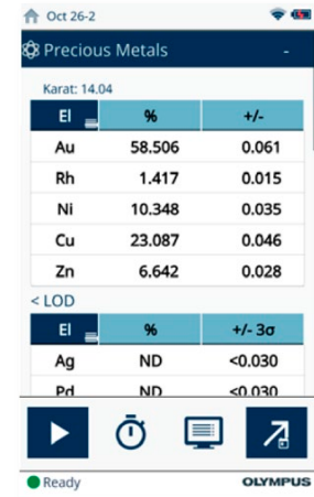
The Vanta analyzer identifies 14 karat gold.
