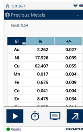
Vanta analyzers alert you if gold plating is possible.
