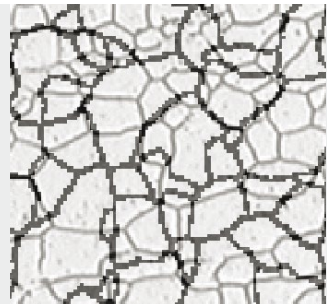
Chart comparison solution (Microstructure with ferritic grains)
