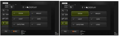
With the desired item selected with the d-pad on the control unit, briefly press the [ENT/MODE] button or click/tap on the tablet to add or remove checkmarks.
