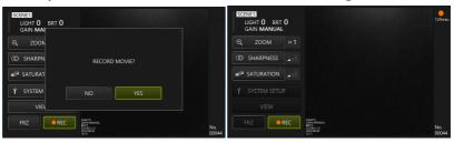
**3.** During recording, click/tap the <REC> button on the tablet to end the recording. In remote control mode, press and hold the [FRZ/REC] button on the control unit.
