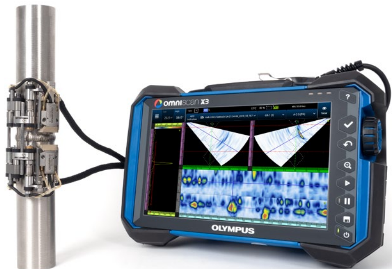
The COBRA scanner on a 0.84 in. pipe with two A15 PA probes with an OmniScan® MX2 16:64 flaw detector displaying two PA groups with sectorial scans and C-scans.
