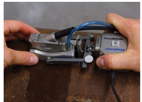
VersaMOUSE and RexoFORM scanners for corrosion inspection.
