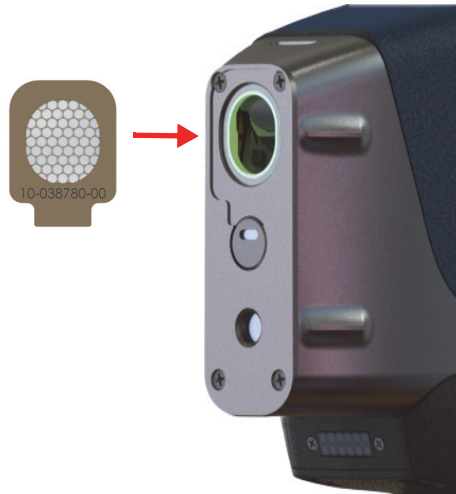
Figure 4-3 New window aligned with probe
