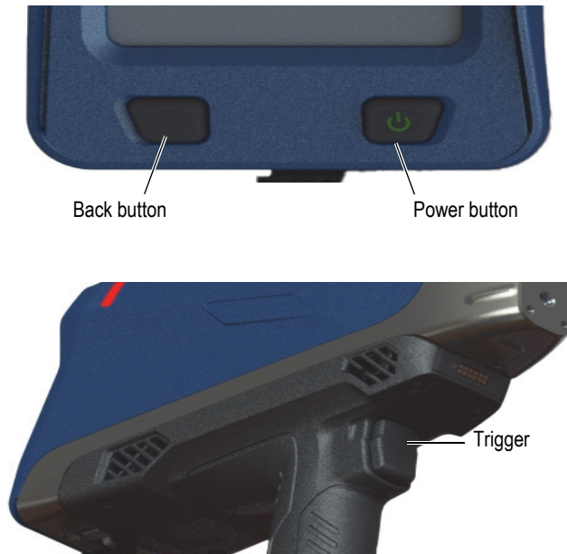
Figure 3-8 Vanta external controls
