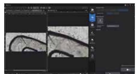
Combine the panorama and EFI functions to obtain large, fully in focus images
