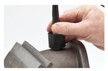
Many cast metal parts or sound-attenuating materials can be measured with the High Penetration software option.
