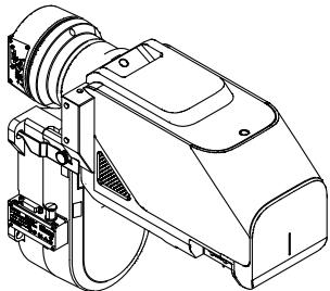
Motorized revolving nosepiece
