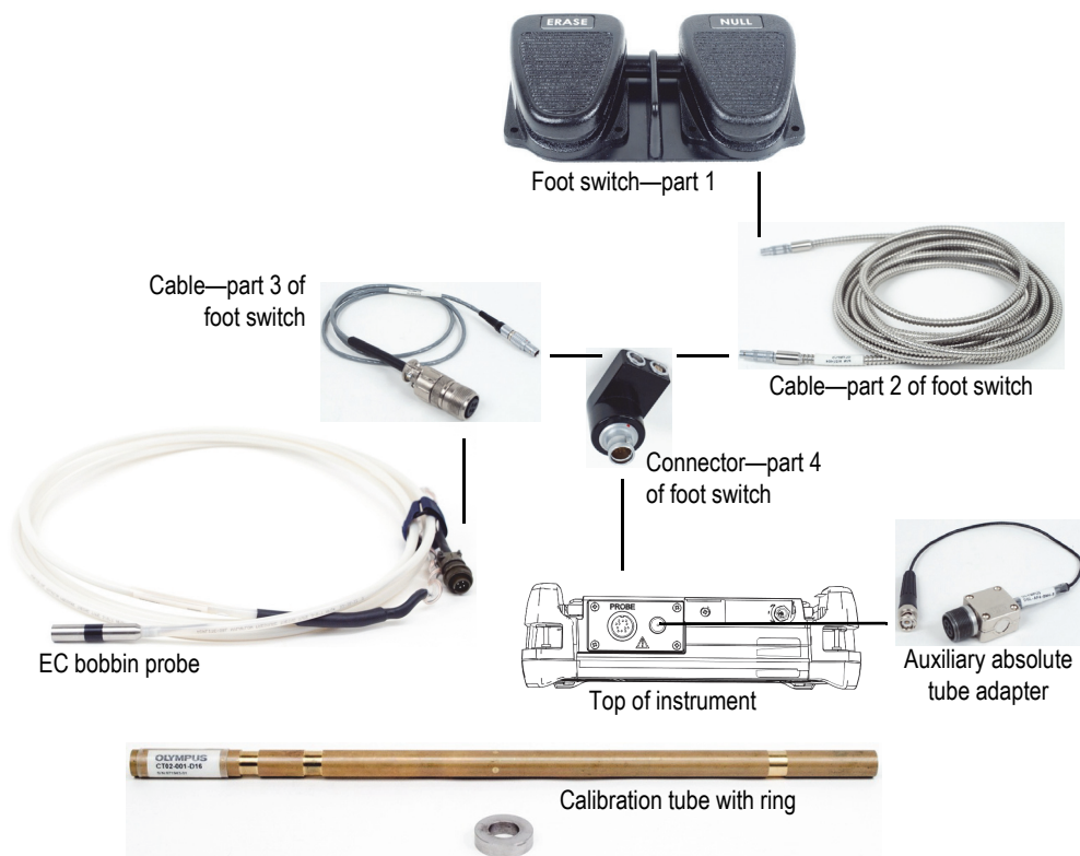
Figure 5-135 Materials—dual frequency for heat exchanger tubing
