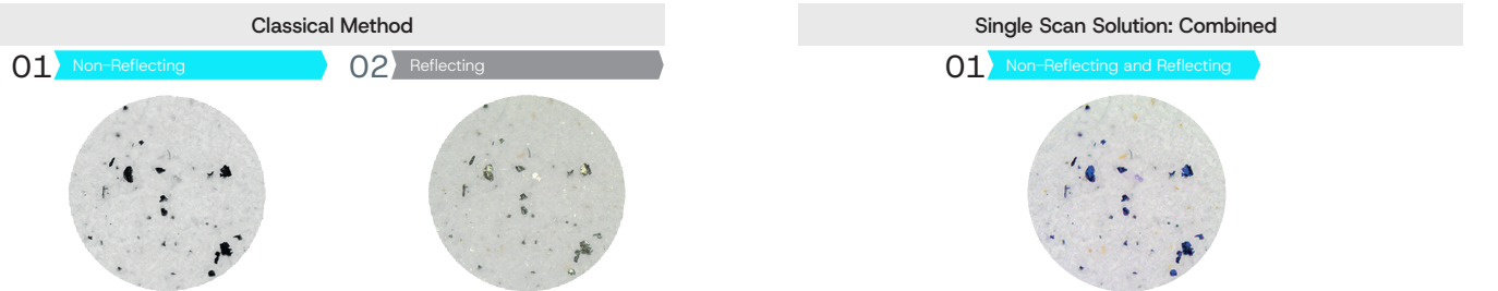
The innovative illumination system separates reflective (metallic) and non-reflective (nonmetallic) particles in a single scan.
